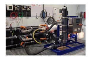
Each filter unit contains a motor-driven, rotating spiral-shaped mechanical cleaning device that continuously cleans collected debris from inside the filter element. Solids are collected at the bottom of the filter housing to be expelled through an automatic purge valve or a continuous concentrate stream.
